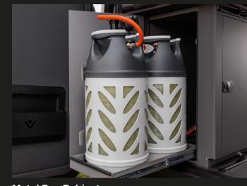
**Metal Gas Cabinet** Space for two large gasolbottles, Duo Control CS and convenient pull-out shelf for easy replacement.
